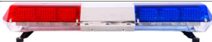
Lightbar HS-1024 DC12V /DC24V/DC12V-DC24V ø5 LED and Halogen bulb(alley lights)/Can With Speaker Full Size:1200*355*222mm (Customized Length) PC Dome/aluminum alloy Base LED/Dome:Amber/red/blue/White/Green
