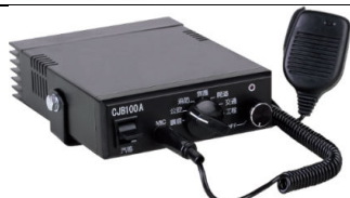
Electronic alarm Siren: CJB-100A 40W/80W/100W 11Ω/8Ω/6Ω/4Ω Over 6 kinds international tones Size(L/W/H):175*139*48mm
