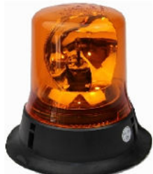
Rotator Beacon HTR-703 DC12V/DC24V/Halogen bulb DC12V-55W/DC24V-70W Mounting:Magnetic Size: \phi 152.4\text{mm} \times \text{H}:177.8\text{mm} Amber,red,blue,White
