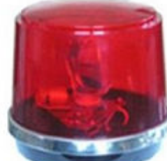
Big Rotator Beacon HTR209 DC12V /DC24V Halogen bulb/25W Mounting:bolt/Magnetic Size: \phi 220\text{mm} \times \text{H}:180\text{mm} Amber,red,blue,White
