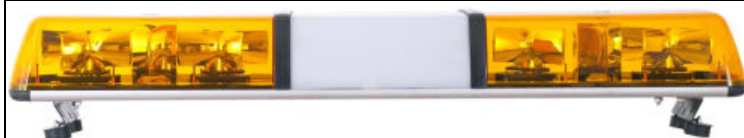
Lightbar HS-1522 DC12V /DC24V/DC12V-DC24V Halogen bulb/Can With Speaker Full Size:1214*296*195mm (Customized Length) PC Dome/aluminum alloy Base Dome Color:Amber/red/blue/White/Green
