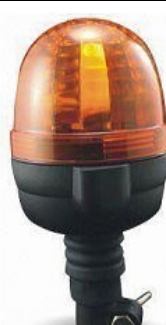
Rotator Beacon HTR-706 DC12V /DC24V/Halogen bulb DC12V-55W/DC24V-70W Mounting:DIN A Pole Size: \phi 110\text{mm} \times \text{H}:217\text{mm} Amber,red,blue,White
