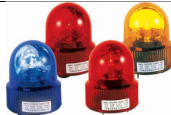
Rotator Bullet Beacon HTR205 DC12V/DC24V Halogen bulb/23W Mounting:bolt/Magnetic Size: \phi 120\text{mm} \times \text{H}:137\text{mm} Amber,red,blue,White
