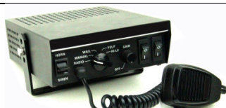
Electronic alarm Siren: CJB-100P 100W/150W/200W 11Ω/8Ω/6Ω/4Ω Over 6 kinds international tones With 2 lamp controllers Size(L/W/H):178*176*85mm
