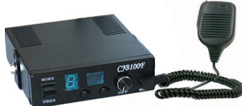
Electronic alarm Siren: CJB-100F 100W/150W/200W 11Ω/8Ω/6Ω/4Ω Digital/Function Display panel Over 6 kinds international tones Size(L/W/H):146*144*38mm
