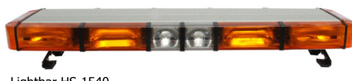
Lightbar HS-1540 DC12V /DC24V/DC12V-DC24V Xenon flash/Can With Speaker Full Size:1220*305*170mm (Customized Length) PC Lens Color:Amber/red/blue/White/Green Aluminum alloy Body:Silvery/Black/White
