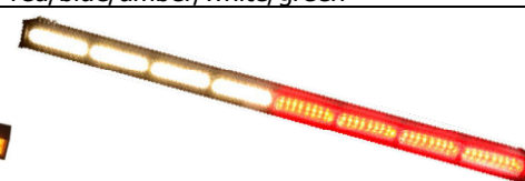
LED Traffic Advisors Lights: HTA-84 DC12V/24V/12V-24V 1W 8LED/LED Modules(1-12pcs Optional) Size: 1040*95*58mm(8pcs LED Module) red/blue/amber/white/green
