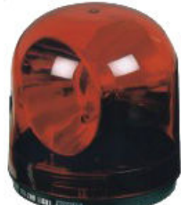
Rotator Beacon HTR-206 DC12V /DC24V Halogen bulb/25W Mounting:bolt/Magnetic Size: \phi 152\text{mm} \times \text{H}:165\text{mm} Amber,red,blue,White
