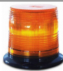
LED Beacon HTL-138 DC10V-30V 3W LEDs/8pcs Mounting:Magnetic/Bolt Size: Ø168mm*H:127.8mm Amber,red,blue,White
