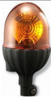
Rotator Beacon HTR-705 DC12V /DC24V/Halogen bulb DC12V-55W/DC24V-70W Mounting:DIN A Pole Size: \phi 141\text{mm} \times \text{H}:255\text{mm} Amber,red,blue,White
