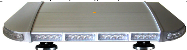
HSM-441 DC12V /DC24V/DC12V-DC24V 1W LED/4pcs LED each module/14pcs modules Size:710*300*98mm(Customized Length) LED/Lens:Amber/Red/Blue/Clear/Green aluminum alloy Body:Silvery/Black/White
