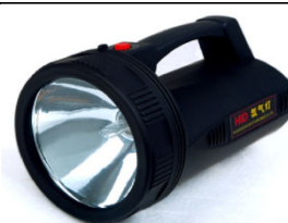
LED/ Xenon Flashlight HLF-05 LED/Xenon Optional Battery:Capacity is 6A Charging time:8h Working Time(Glare/ Faint): Xenon:2h/4h, LED:16h/20h Light Size: ø125mm*L:200mm
