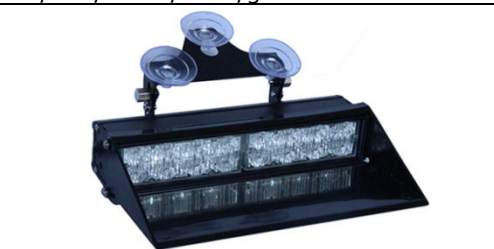
LED Visor Windshield Light: HV-281 DC12V /DC24V/DC12V-DC24V/ 1W LED Size(L/W/H):118mm×143mm×49mm red/blue/amber/white/green
