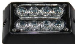
LED Flashing Light: HF-244 DC12V/24V/12V-24V 3W LED/8LED Size:115mm*75mm*27.5mm red/blue/amber/white/green
