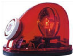
Rotator Snail Beacon HTR210 DC12V /DC24V Halogen bulb:23W with siren Mounting:Magnetic Size: 182\text{mm} \times 124\text{mm} \times 135\text{mm} Amber,red,blue,White
