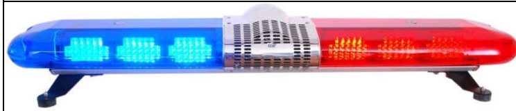
Lightbar HS-1020 DC12V /DC24V/DC12V-DC24V ø5 LED /Can With Speaker Full Size:1210*314*142mm (Customized Length) PC Dome/aluminum alloy Base LED/Dome:Amber/red/blue/White/Green
